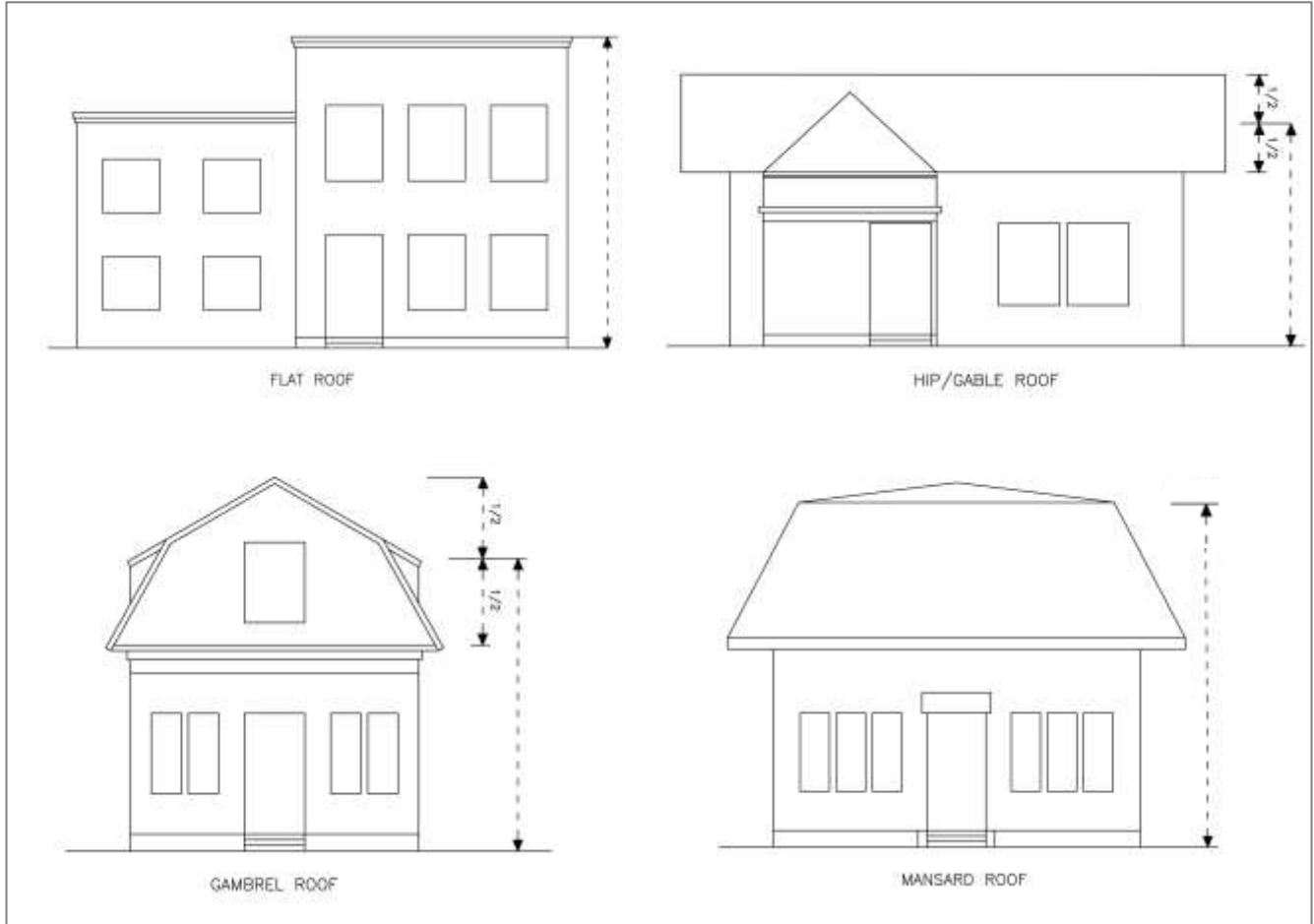
Exhibit 7-3. Measurement of building height
